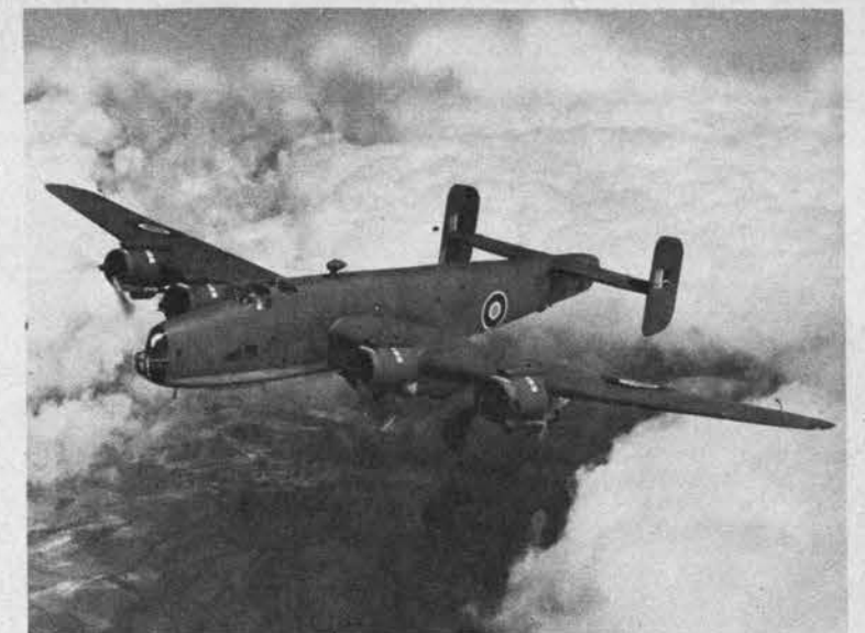
Fast Halifax transport parallels the Lancastrian, a similar reworking of Lancaster bomber design. Streamlined cone replaces tail turret.
